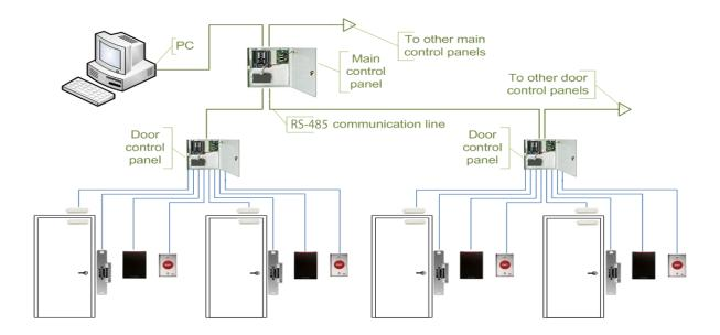
Access Control Systems Using Serial Main Controller and Intelligent Readers
